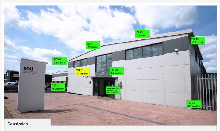
'ARGUS' is an easy-to-use software suite with a graphical user interface (GUI) that allows quick and easy interpretation of large amounts of instrumentation data from a variety of sources.
