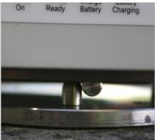
For Horizontal Tilt-Plates, place the Tiltmeter on the Tilt-Plate and ensure that the locating bars touch the protruding rounded studs on the Tilt-Plate *in both directions* (see photos above).
