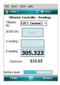
The User Screen shows a Battery Level bar. Once a reading has been taken (in other words, data have been sent back from the reel), the user screen will show this bar indicating the reel battery level. The bar's start and end voltages are 13v (right hand end) and 11v (left hand end). It does not change colour at all – the indication of the state of the battery is the position of the bar.
