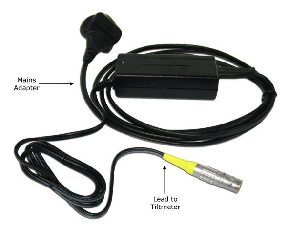
To charge from the mains, plug the Lemo plug (sleeved plug pictured above and below) into the socket in the centre of the reel hub, ensure the system is turned off and then connect
