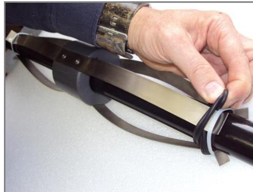
Wrap the long section of the rubber band over the spring legs and back to meet the short end.
