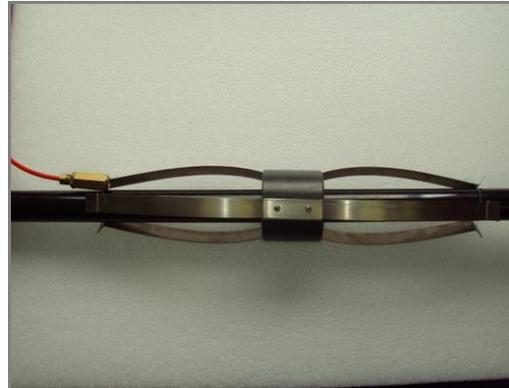
Ensure that the three round apertures, in the main body of the spider magnet, indicating the location of the target's magnets, will be facing upwards when the spider magnet is installed in the ground and that the pneumatic cutter is incorporated into the upper loop of nylon line.
