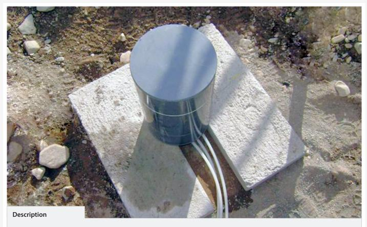
The Hydraulic Overflow Settlement Cell is used for measuring vertical movements and controlling subsidence.
